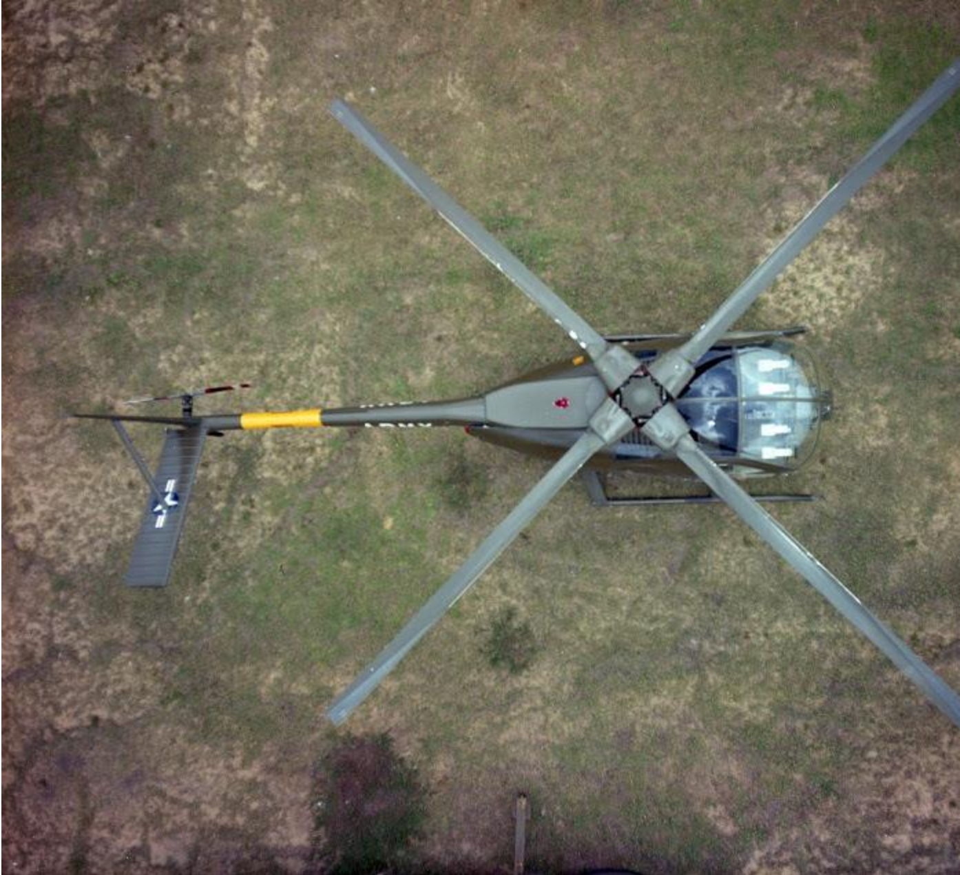
Interesting overhead photograph of a Hughes YOHO-6. Note the blade cuffs. (U.S. Army)
